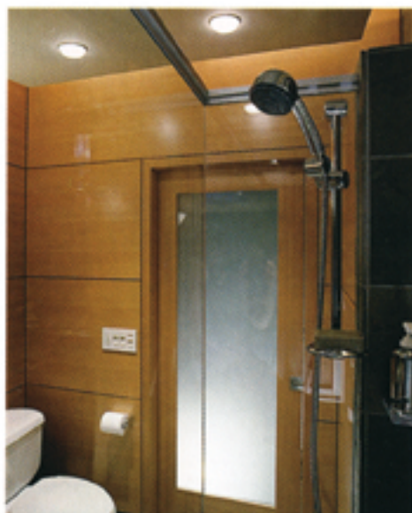
Meticulous layout and clean lines. At the bathroom's entry, a pocket door with frosted-glass panel admits light from the hall. Lights above the false ceiling illuminate the walls' tops. Photo taken at B on floor plan.
